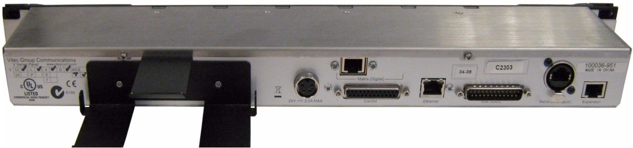
Figure 13: Completed Rack Mount Panel Upgrade with T-Adapter
