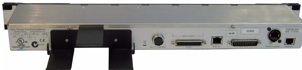
Figure 4: V-Series Rack Mount Panel with PSU Removed
